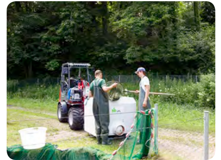
The compressor attached to the right side of the machine supplies air to the fish in the water tank.
